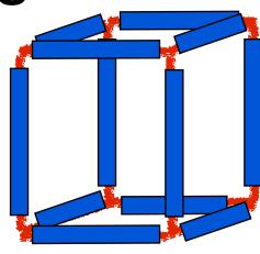
Bubble frame made from pipe cleaners inside straws
